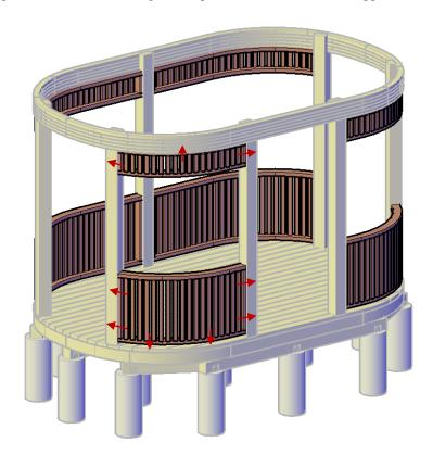
**Step 9:** Attach the braces to the posts with 3/8" x 8" bolts ( $\rightarrow$ ) and 3/8" x 10" bolts ( $\rightarrow$ ).
