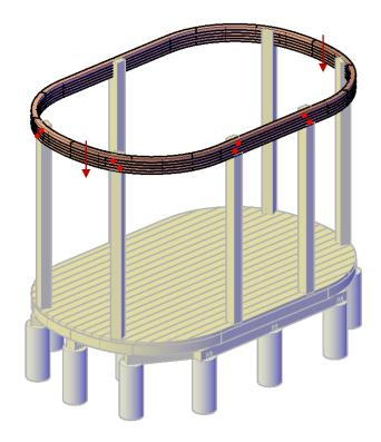
**Step 8:** Use 5/16" x 3" lag bolts to attach the railings to the posts, the floor and to the supports.
