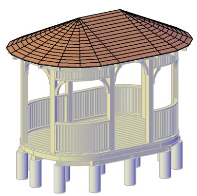
**Step 13:** Use 4" deck screws to attach covers to the roof boards.
