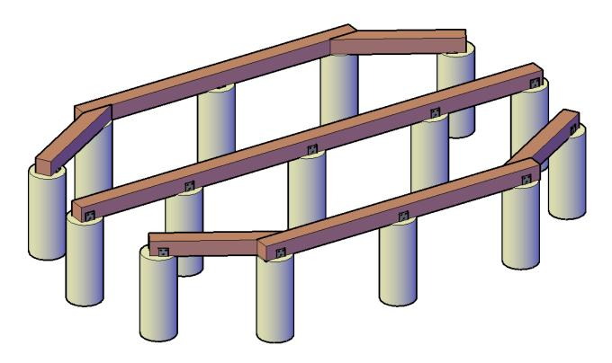
**Step 4:** Assemble the frame floor with 3" deck screws.
