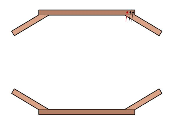
**Step 3:** Attach the floor supports to the L-Brackets with  $5/16^{\prime\prime}$  x  $3^{\prime\prime}$  Lag Bolts.
