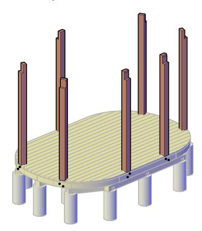
**Step 7:** Attach the supports to the posts with  $3/8^{\prime\prime}$  x  $5\frac{1}{2}^{\prime\prime}$  bolts (•). The supports will be attached together with  $3/8^{\prime\prime}$  x  $8^{\prime\prime}$  bolts (-).
