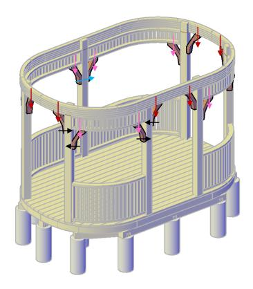
**Step 10:** Attach rafters to the supports with 3/8" x 10" ( $\rightarrow$ ) and 3" deck screws. After that, attach to the ridge beam with 3/8" x 6" lag bolts ( $\rightarrow$ ).
