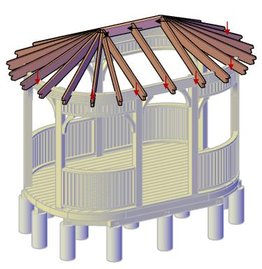
**Step 11:** Use 1 5/8'' deck screws to attach the roof boards T&G to the rafters.
