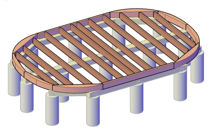
**Step 5:** Attach the floor boards with 2 ½ ' deck screws.
