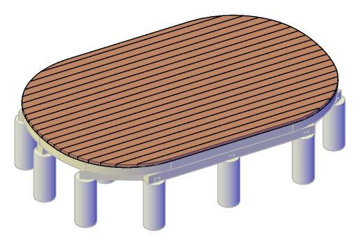
Step 6: Use 3/8" x 4" lag bolts to attach the posts to the floor.
